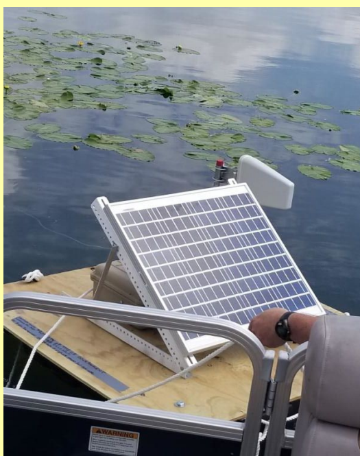
Solar panel that powers underwater cameras.
