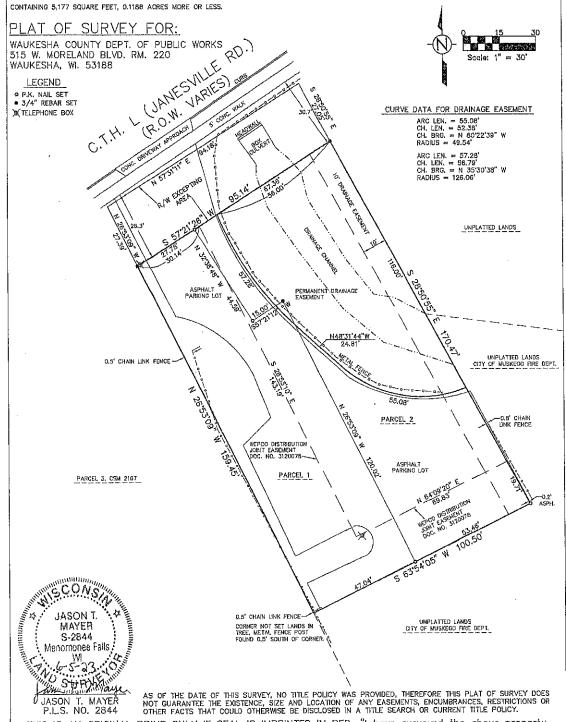
THIS IS AN ORIGINAL PRINT ONLY IF SEAL IS IMPRINTED IN RED. "I have surveyed the above property, and the above map is a true representation thereof and shows the size and location of the property, its exterior boundaries, the location and dimensions of all structures thereon, fences, apparent easements, roadways, and visible encroachments and is in compliance with Wisconsin Administrative Code AE-7 for property survey standards and is correct to the best of my knowledge and belief.
