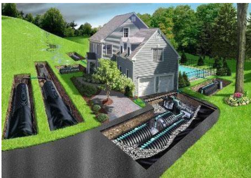
Infiltration chamber - Image: tetoomey.com
