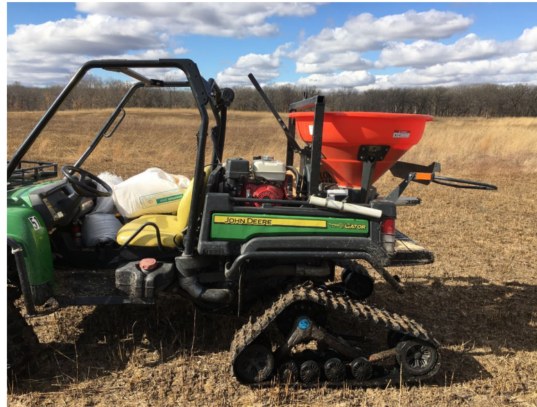
Typical native seed installation equipment
