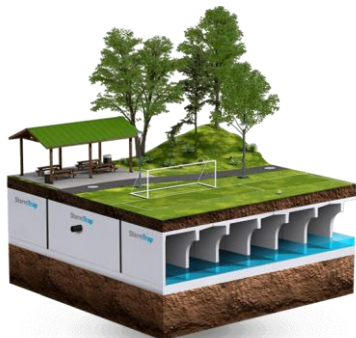
Underground wet detention basin
