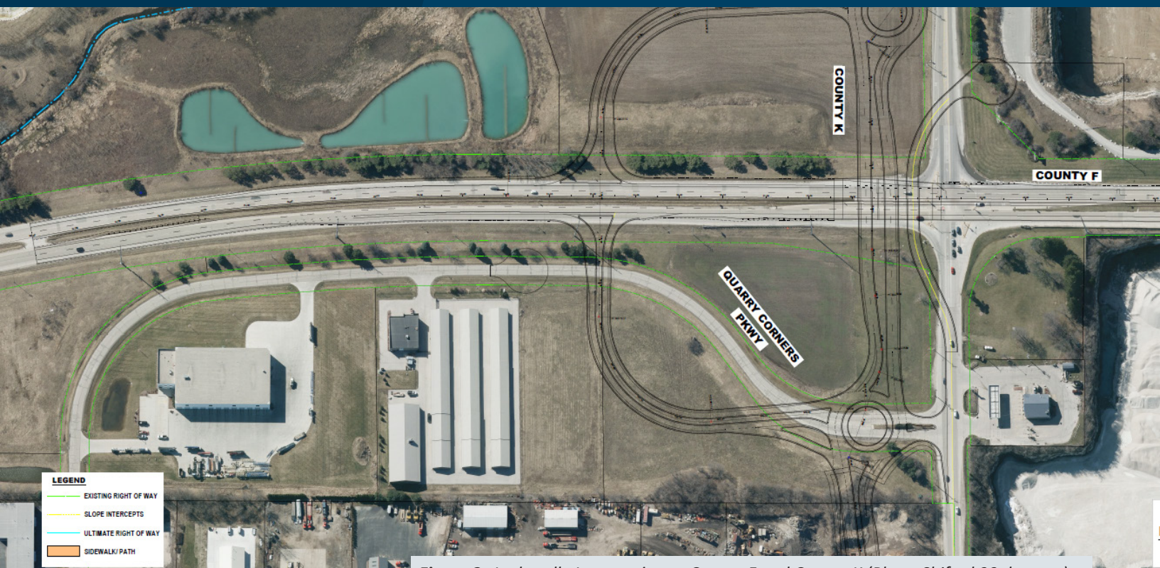
Figure 2: Jughandle Intersection at County F and County K (Photo Shifted 90 degrees)
