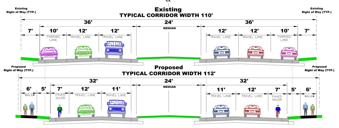
\*The design team is considering options of sidewalk on one or both sides of the roadway. The recommended alternative may be a hybrid (mix) of the alternatives shown which would result in a different configuration for northbound and southbound Moorland Road.
