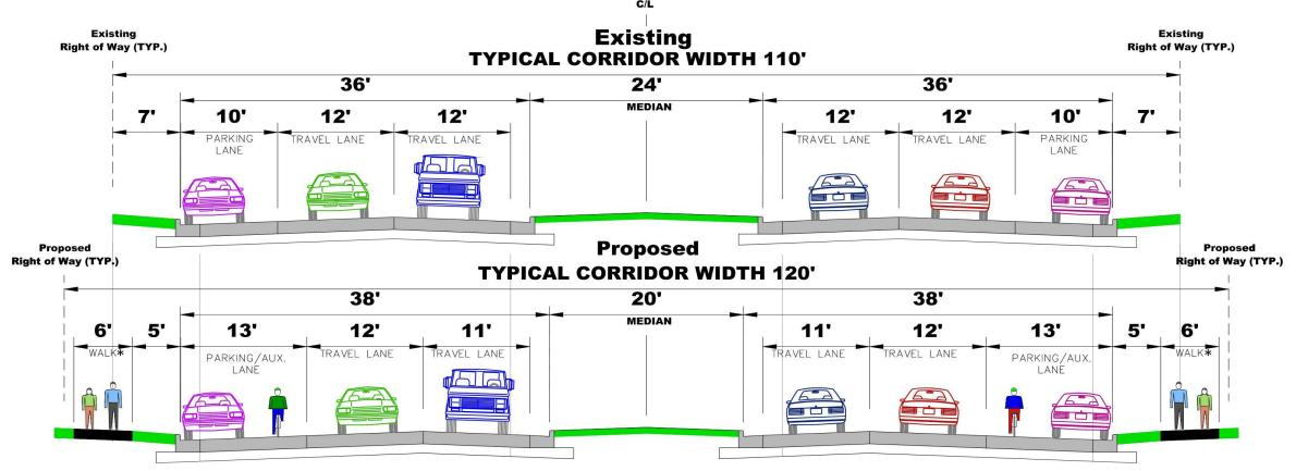
\*The design team is considering options of sidewalk on one or both sides of the roadway. The recommended alternative may be a hybrid (mix) of the alternatives shown which would result in a different configuration for northbound and southbound Moorland Road.
