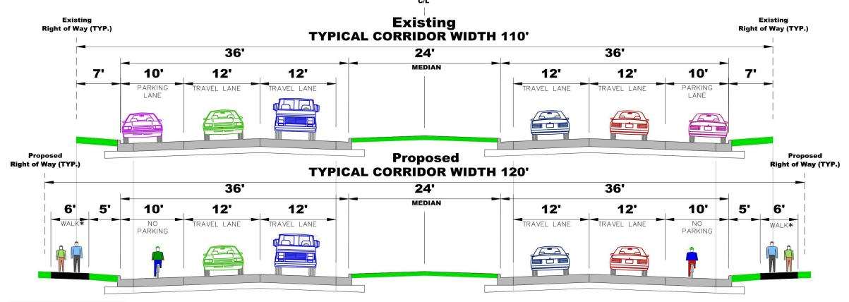
\*The design team is considering options of sidewalk on one or both sides of the roadway. The recommended alternative may be a hybrid (mix) of the alternatives shown which would result in a different configuration for northbound and southbound Moorland Road.
